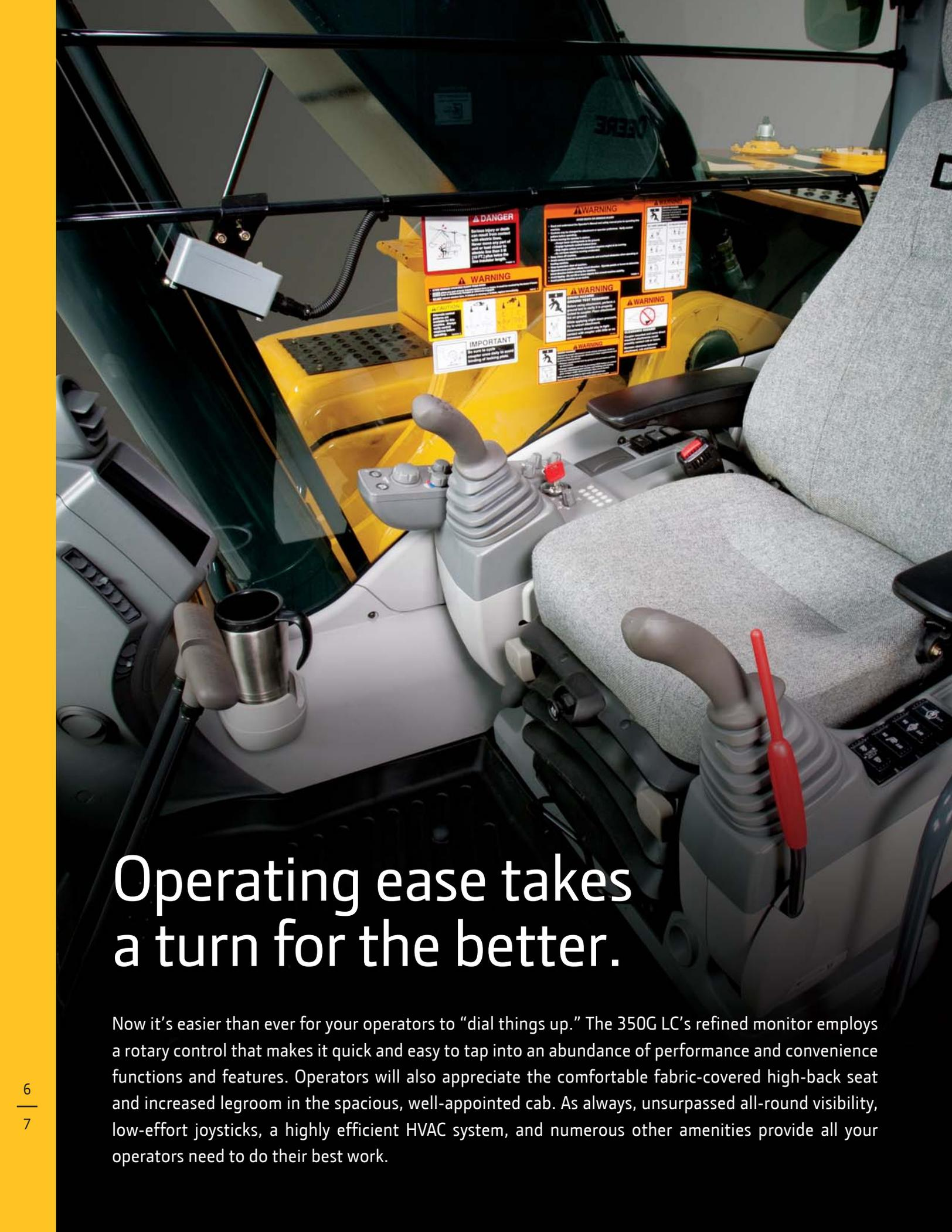
The image shows the interior of a John Deere 350G LC tractor cab. The operator's seat is a grey fabric-covered high-back seat. In front of the seat is a control panel with two joysticks, a gear selector, and various buttons. A stainless steel mug is in a holder on the left. The dashboard features a monitor with a rotary control. Several warning and important labels are posted on the dashboard. The overall design is functional and ergonomic.
